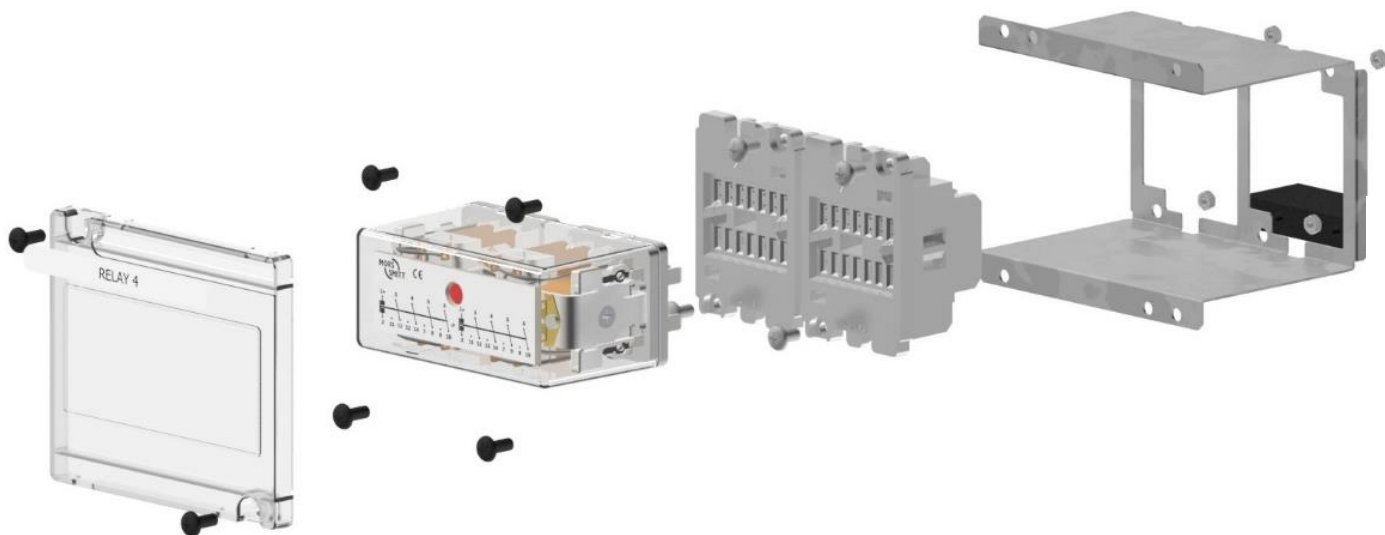
Figure 6: Exploded view of the size 4 element kit
