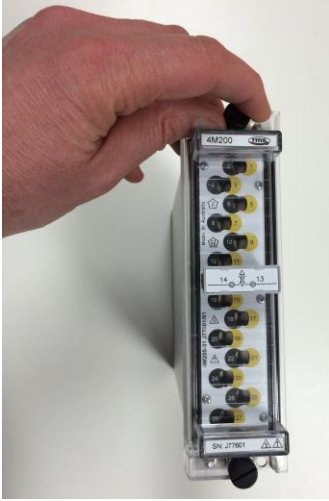
Undo Front Cover Thumbscrews to allow Front Cover Removal
